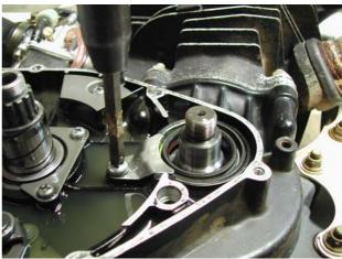
**9.** Remove crankshaft seal with seal pick tool being careful not to mark or damage any surfaces.
