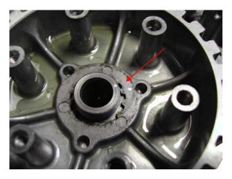
**8.** Now you can remove the primary drive gear, primary drive gear key and then undo crankshaft seal retaining tab bolt/s.
