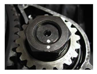
**7.** Again, more fitting marks are required to ensure parts are reassembled as they were. Remove clutch driven hub. Ensure thrust washer behind it and any bushes, spacers or bearings are not lost or damaged.
