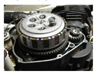
**3.** If not already marked, mark the clutch cover assembly so it goes back together the same way. A white paint pen is useful for this. In the following image, the manufacturer has been kind enough to
