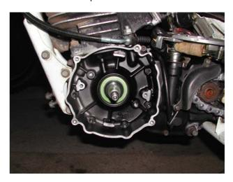
Reassemble in reverse order using a torque wrench to tension rotor nut. Please contact TRIALTECH if you have any questions - 0437 213 550.
