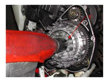
**6.** Mark the primary drive gear and shaft and remove nut.
