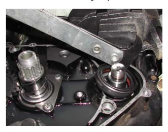
**10.** Install new seal with a suitable seal driver. Ensure seal is 'driven' in uniformly and seats to where the position of the worn seal was.
