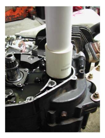
**11.** Lubricate the seal lightly with the same 2-stroke oil you use in your fuel/oil mix. Now assemble in reverse order steps 9-1. Make sure you use a torque wrench to tension the nuts. If torque wrench not available, tension until the marks you have made re-align. A folded rag is useful for 'jamming' the primary drive gear teeth. A two cent piece (if you can find one) is also useful as the material won't damage the drive teeth.
